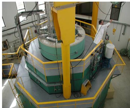
**FIGURA 10. CONSOLA DE CONTROL Y RECINTO DEL REACTOR IAN-R1**
